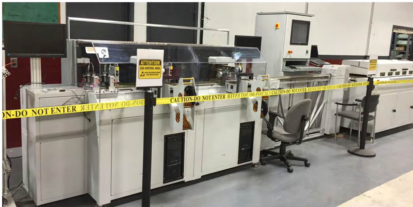
Figure 1: In-line paste-place-reflow system to mount parts from reel to reel.
